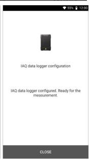
Following successful configuration, the testo 400 can be disconnected from the IAQ data logger. The measurement starts at the defined time or as soon as the setup has been completed (if the start time has been set to manual). The green LED on the IAQ data logger flashes rapidly at short intervals.
