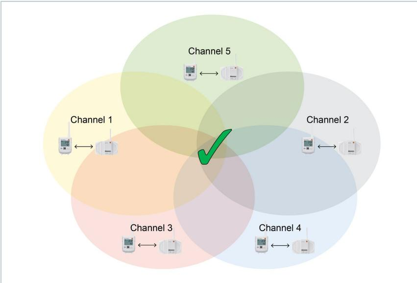
**5.3** If all 5 channels are already in use, the gateway/base selects the channel that the channel selection started with.
