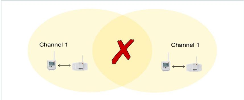
The more loggers communicate on the same channel within radio range, the higher the probability of radio communication interference, which can result in "connection missing" alarms.
