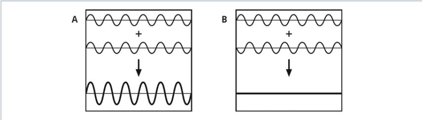
Erasure is often caused by a reflection of the radio wave on different surfaces. The reflected wave is out of phase or offset with respect to the transmitted radio wave, thus causing an erasure.
