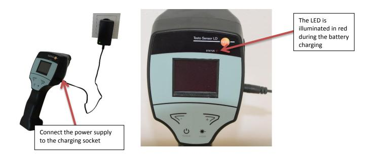
The TESTO SENSOR LD checks the charge status of the battery and automatically starts the charging process. The following scenarios are possible:
